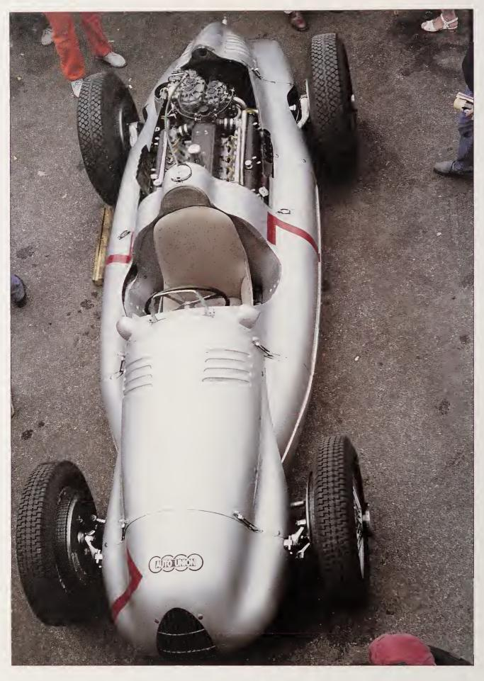
The Auto Union as it first appeared in 'A' form in 1934, when its unorthodoxy baffled the racing world. Some of the air scoops on this car appear to have been additions after trials, and the nationalistic emblem was seldom carried outside Germany after hostile receptions. An external starter engaged the shaft projecting at the rear.
