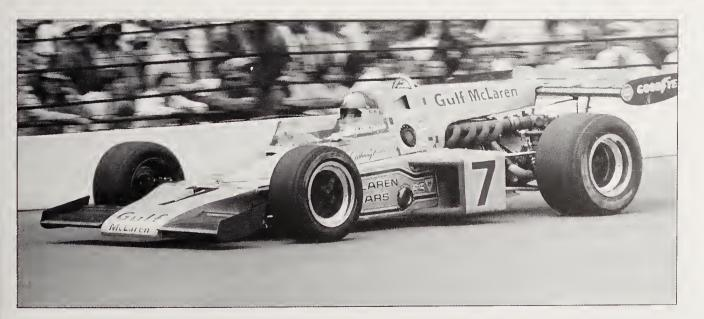
Johnny Rutherford in a works M16C in 1973. This variant has an odd engine cover merging into the rear wing, and the radiator shrouds have been revised. Rutherford took pole, but was only ninth in the race.
